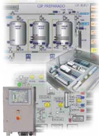
Otomatik PLC kontrollü paneller Automation: PLC, control panels, etc.
